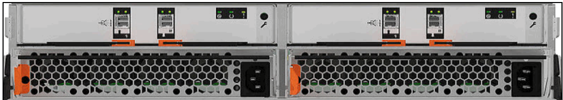
Figure 15 Rear view of IBM FlashSystem 7000 Expansion Enclosure Model 12G
