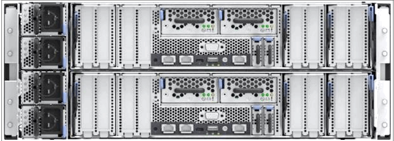
Figure 15 Rear view of IBM FlashSystem 9500 control enclosure
