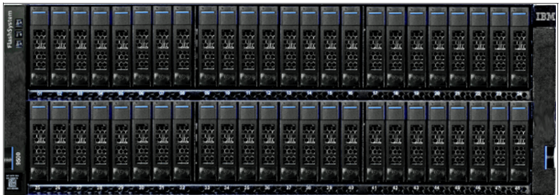
Figure 2 IBM FlashSystem 9500 control enclosure front view
