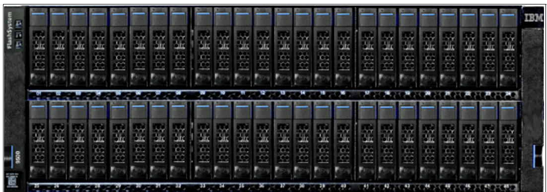
Figure 13 IBM FlashSystem 9500 control enclosure front view
